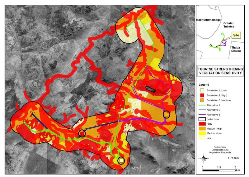
Figure 10: Composite sensitivity map for the proposed corridors and substation alternative sites
